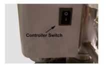
To remove the battery for charging and/or scooter transport you should first turn the controller switch to the off position. Then using two hands, grab the battery on each end and lift it straight up. The battery extends slightly beyond the battery platform to provide an easy way to grasp the battery pack.
