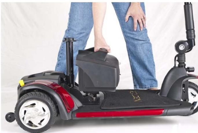
**Figure 22. Battery Pack Installation**
