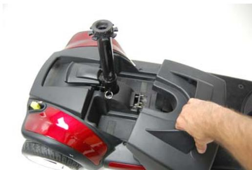
**Figure 16. Removing the Battery Pack**
