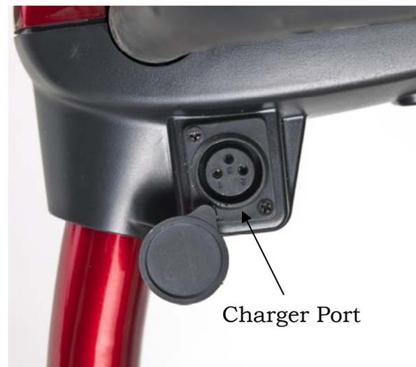
**Figure 27. Charging Batteries**
