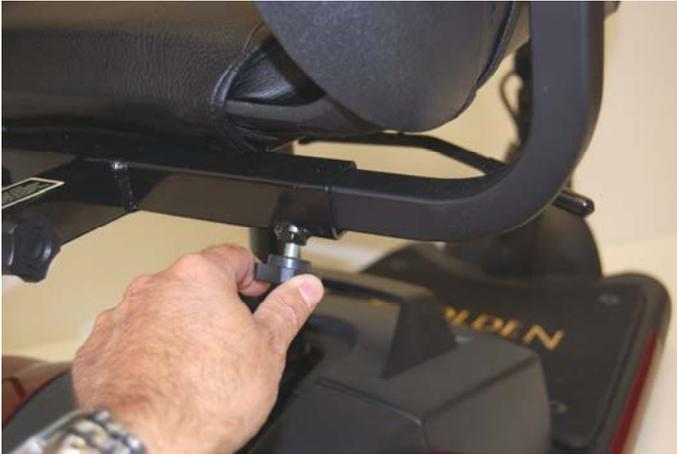
**Figure 6. Armrest Width Adjustment**
