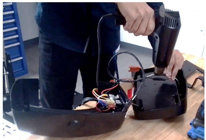
Fig. 8: Using a heating element to tighten the heat shrink.
