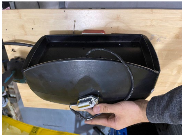
Fig. 10: Hang the extension cord and light over the back of the motor head cover.
