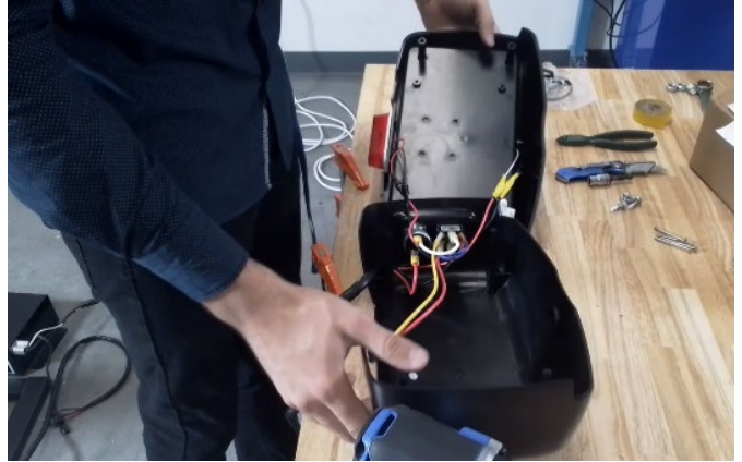
Fig. 6: Separation of motor head revealing license plate light wiring.
