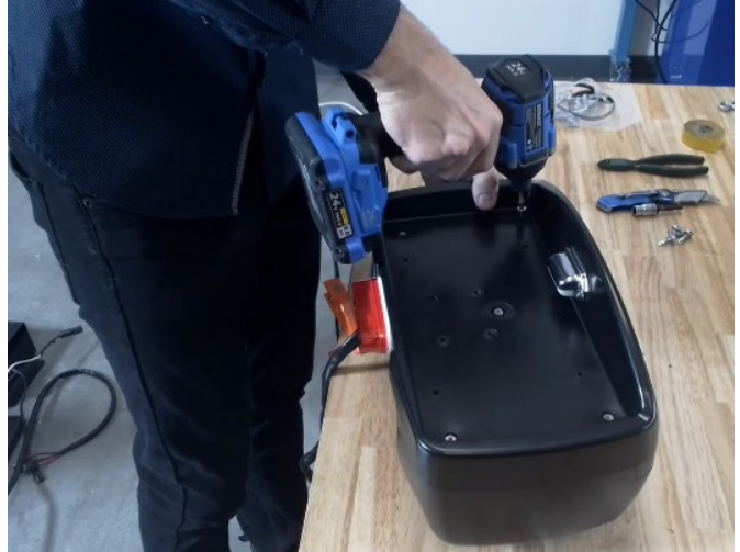
Fig. 4: Using a drill to remove Phillips head screws.
