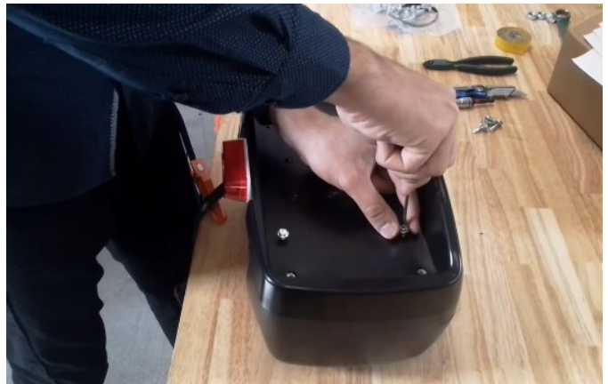
Fig. 5: Using a screwdriver to remove license plate screws
