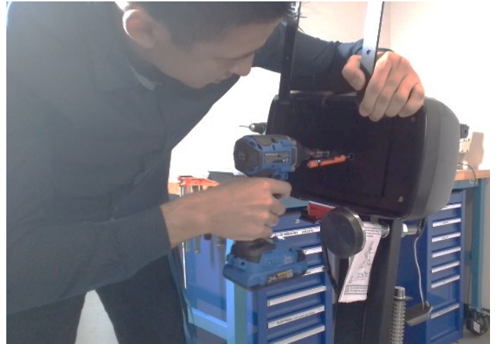
Fig. 12: Use a drill to mount the motor cover and license plate riser.
