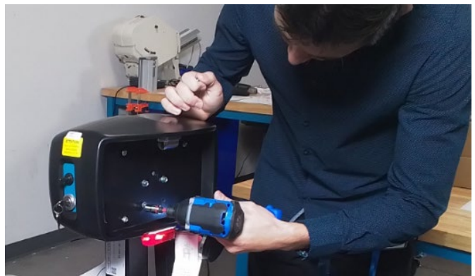
Fig. 3: Using a drill to unfasten the motor head from the bracket.
