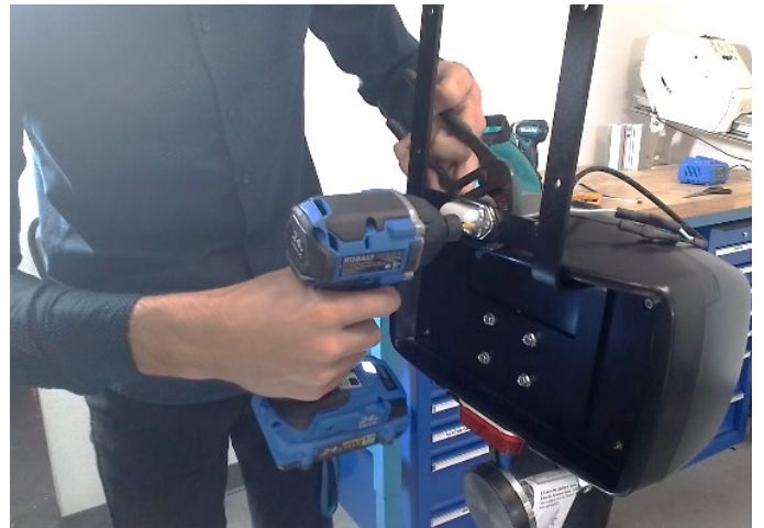
Fig. 13: Use a drill to mount the license plate light.
