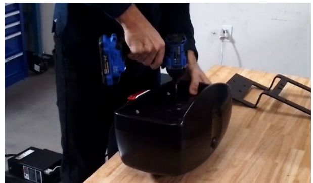
Fig. 11: Using a drill, reassemble the motor cover.
